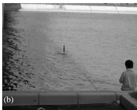
Fig. 3 Moving aDcp across the Gion diversion channel using a piece of rope (a) a close view and (b) a far view
