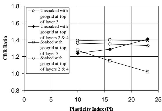
Fig. 6 CBR ratio in soaked and unsoaked tests with different kinds of reinforcement
