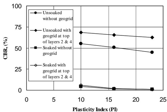
Fig 3. CBR values for various PIs with geogrid in 2 layers
