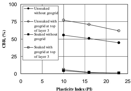
Fig. 2 CBR values for various PIs with geogrid in layer 3
