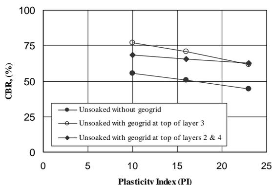
Fig. 4 Comparison of different kinds of reinforcement in CBR tests for various PIs
