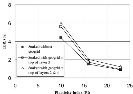
Fig. 5 Comparison of different kinds of reinforcement in CBR tests for various PIs
