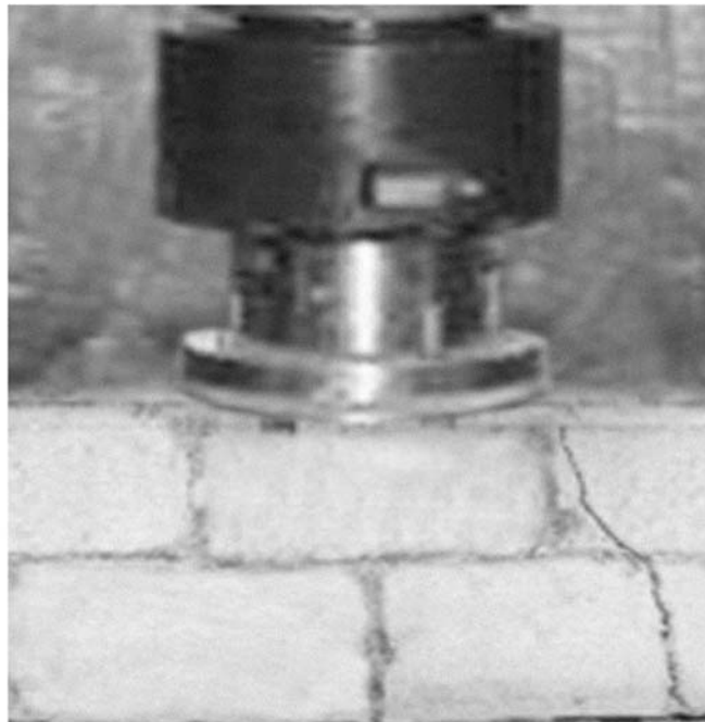
Fig. 3 Shear Failure for Beam Tests
