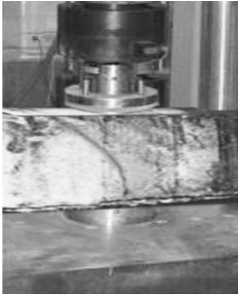
Fig. 4 Shear Failure of Beam with GFRP
