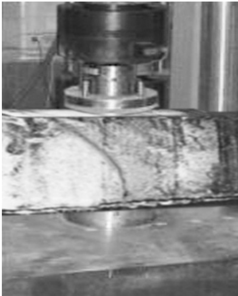
Fig. 4 Shear Failure of Beam with GFRP
