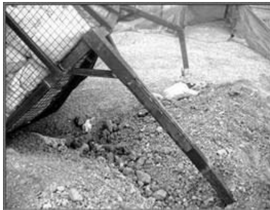
Fig. 3 The collapsed initial steel frame under a gravity load of 30,000 kgf
