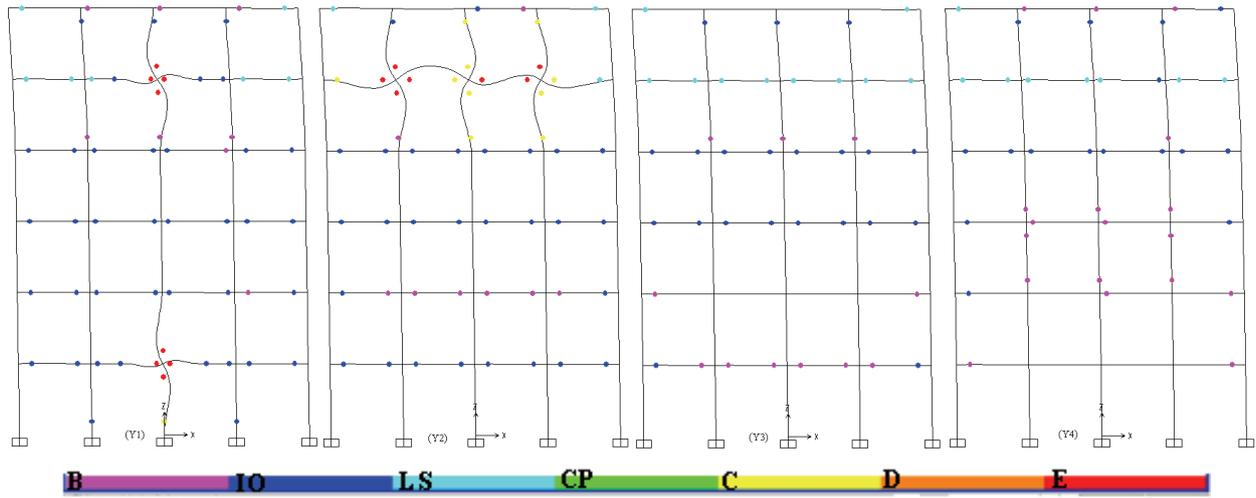
Fig. 2. Plastic hinge formation status in 6 story building under Tabas excitation with PGA=0.7g
