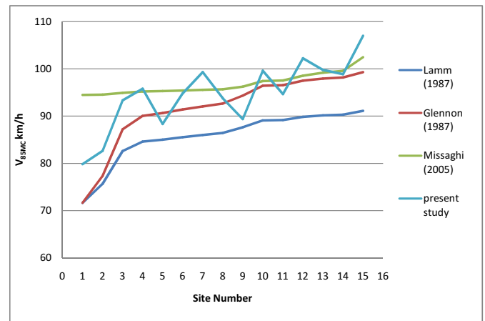
Fig. 6. Comparison of the predicted values of V_{85MC} from model developed in this study and with those from previous research
