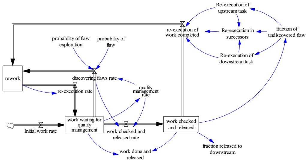
Fig. 5 Conceptual diagram of quality management process model
