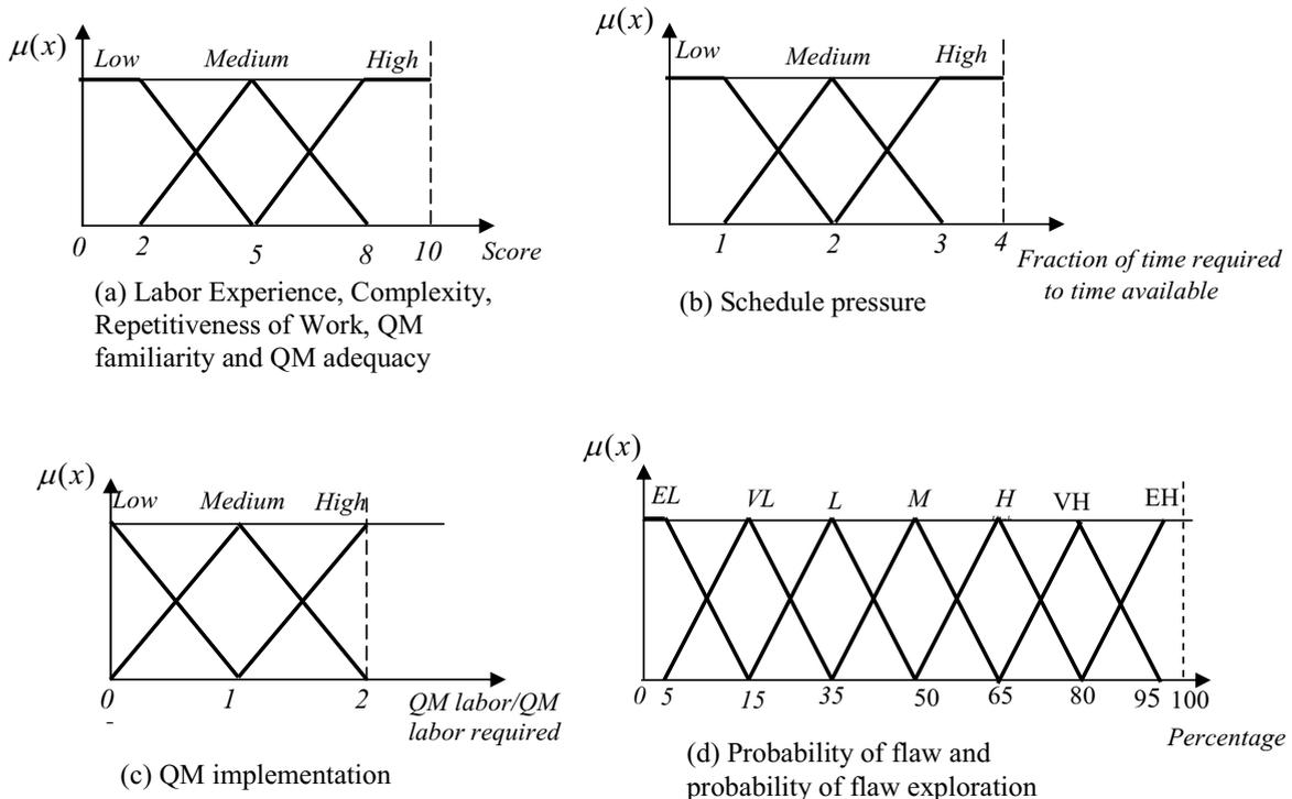
Fig. 4 Membership functions of different factors affecting the QM process
