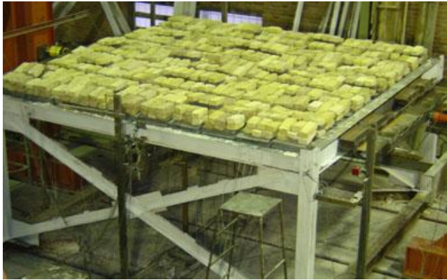
Fig. 8 Gravity loading by lead blocks and additional bricks in the 1 st specimen
