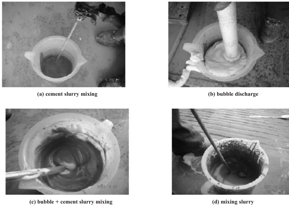
Fig. 3 Lightweight ATS production process
