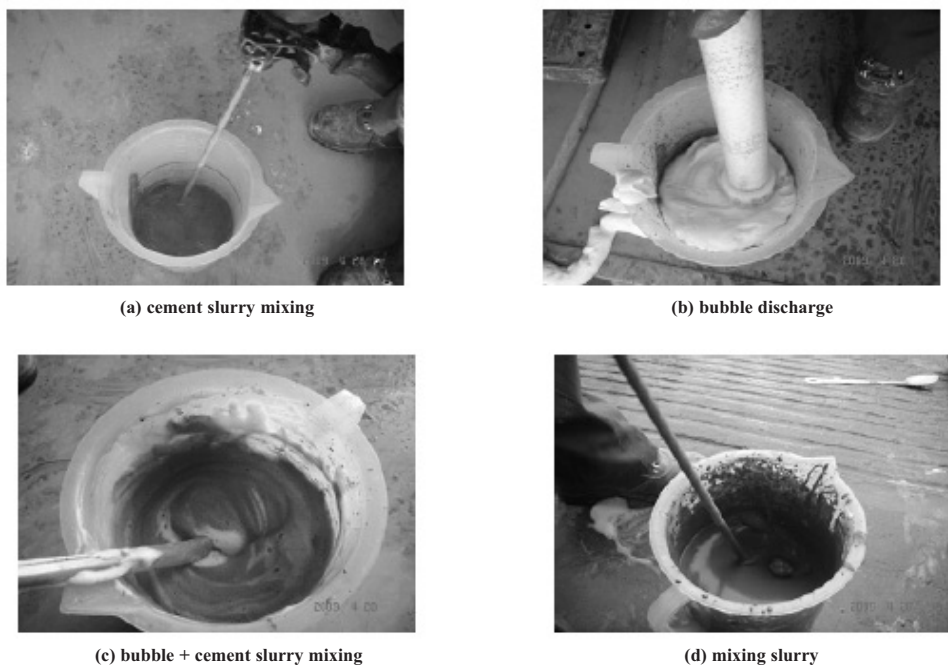
Fig. 3 Lightweight ATS production process
