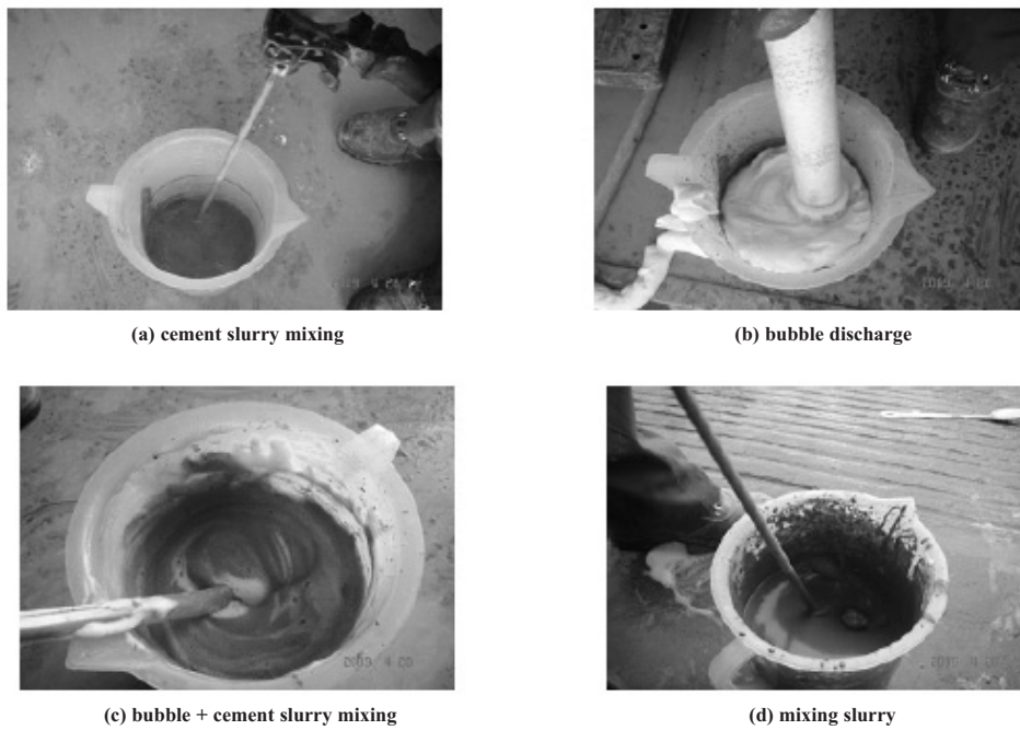
Fig. 3 Lightweight ATS production process
