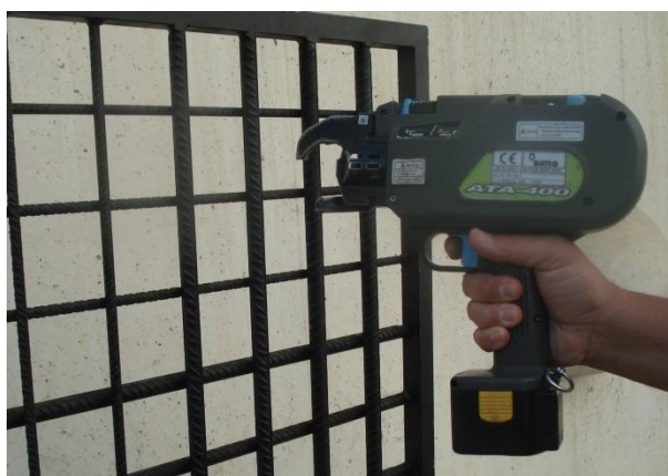
Fig. 6 Battery powered rebar tier
