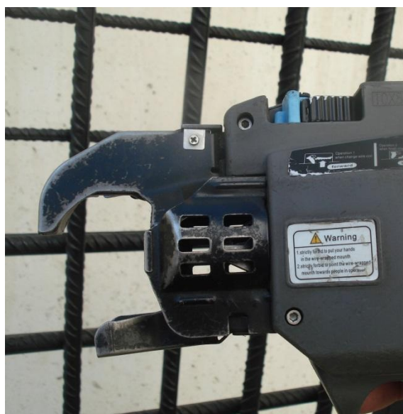
Fig. 4 Close-up of the adjustable pick
