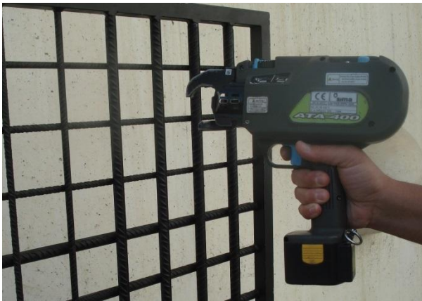
Fig. 6 Battery powered rebar tier
