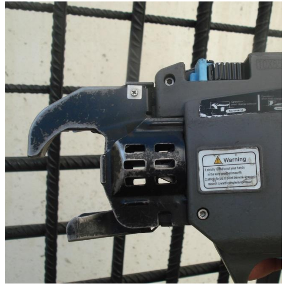
Fig. 4 Close-up of the adjustable pick
