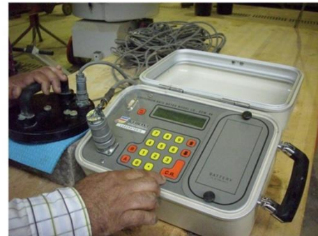
Figure 4 GECOR-8 (Corrosion Measurement device)
