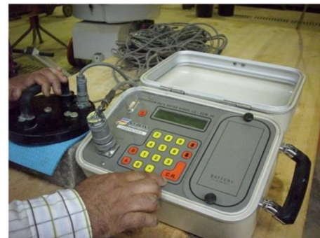
Figure 4 GECOR-8 (Corrosion Measurement device)
