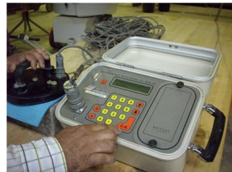
Figure 4 GECOR-8 (Corrosion Measurement device)
