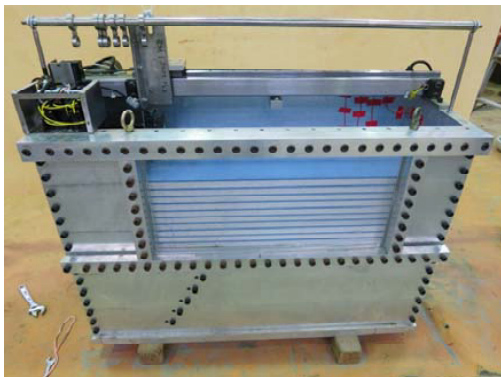
Fig. 1 Fault simulation container
