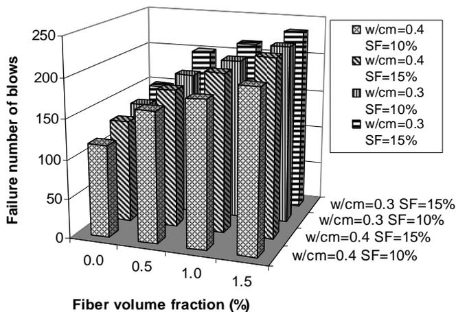
Fig. 6 Impact (ultimate failure) characteristics at 56 days of HPSFRC (w/cm = 0.4 & 0.3)
