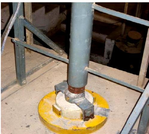
**Fig. 1** Disc specimen under drop weight impact test
