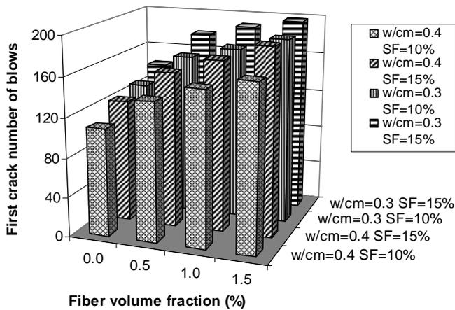
Fig. 5 Impact (first crack) characteristics at 56 days of HPSFRC (w/cm = 0.4 & 0.3)
