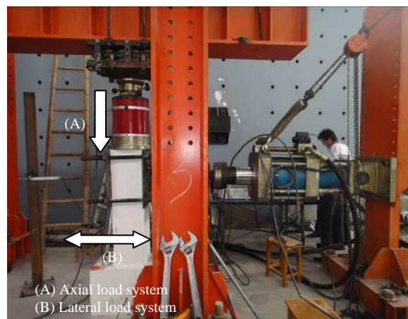
Fig. 3 Test set-up for cyclic loading test
