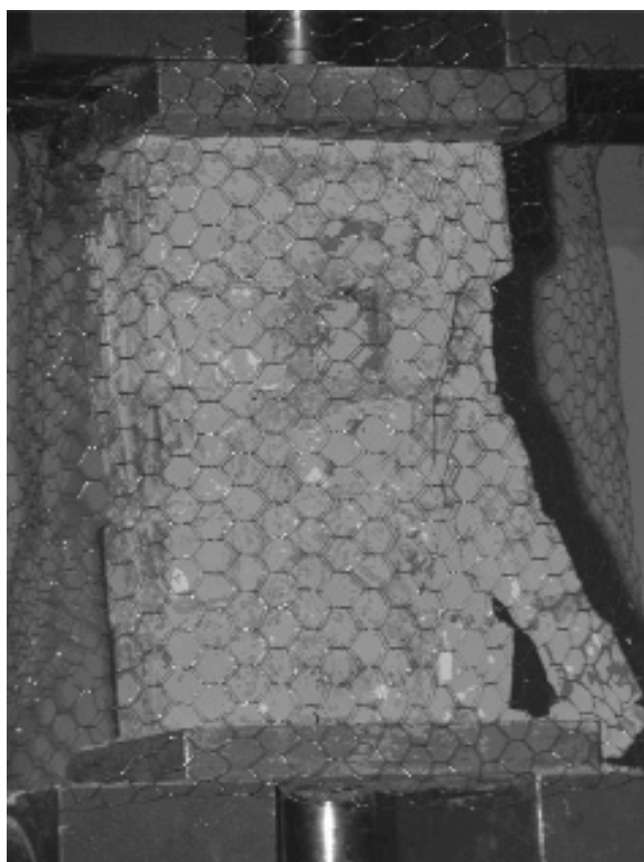
Fig. 6 Cracking and failure development in masonry sample No.3 at last loading step
