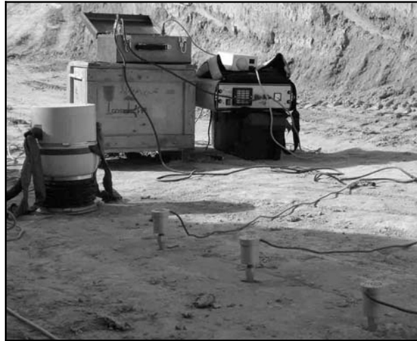
Fig. 3. Surface wave attenuation measurements at the site
