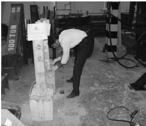
Fig.8 Cleanig surface of the damaged columns
