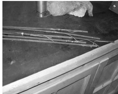
Fig.4 Strain gauges were installed on the bars
