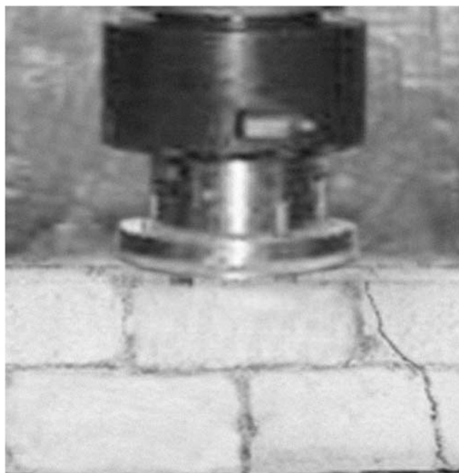
Fig. 3 Shear Failure for Beam Tests
