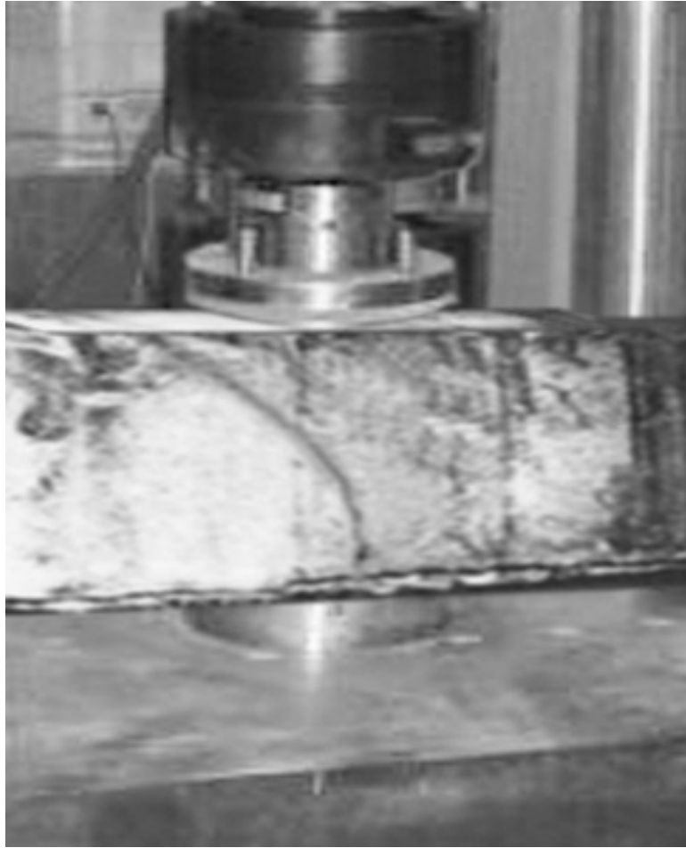
Fig. 4 Shear Failure of Beam with GFRP
