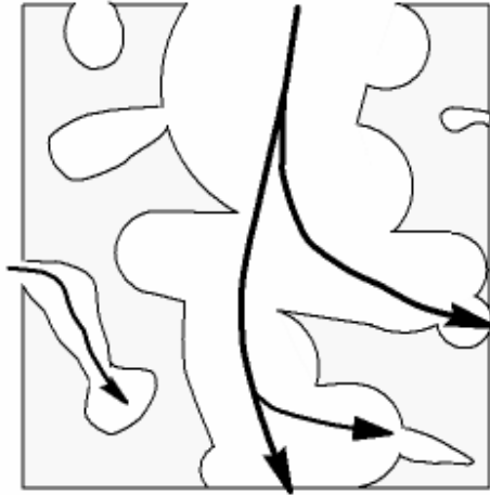
Fig.1 Flow through a typical porous specimen.
