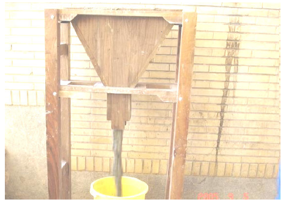
Fig. 4. V-funnel test of SCLWC
