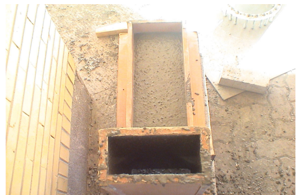
Fig. 5. L-box test of SCLWC
