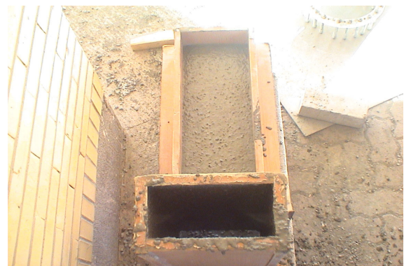
Fig. 5. L-box test of SCLWC
