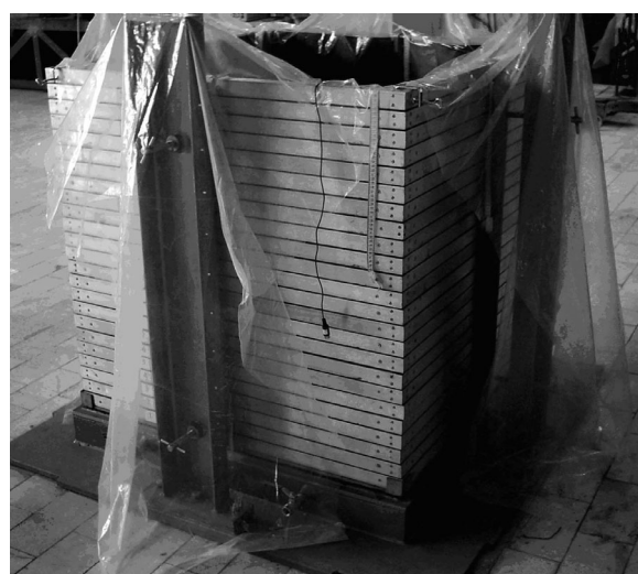
Fig.2. Laminar shear box
