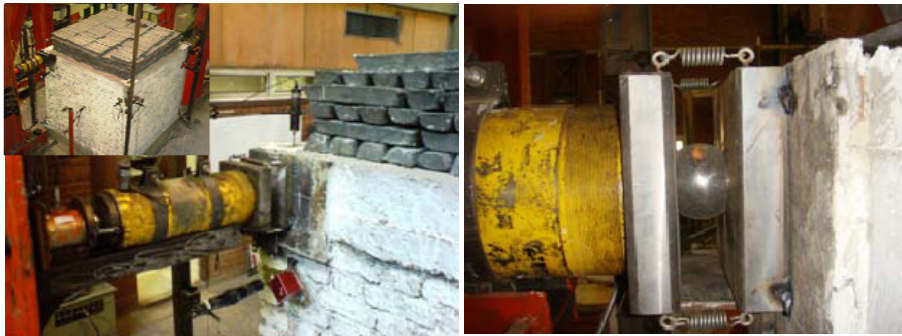
b) Application of loading system
