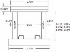
Fig. 2 two-span bridge bents [1]
