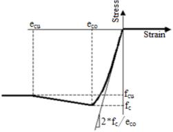
Fig. 3 Concrete01 Material Parameters [7]
