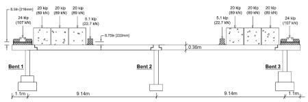
Fig. 1 Elevation and top view of two-span bridge [1]
