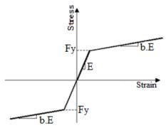
Fig. 4 Steel01 Material Parameters [1]
