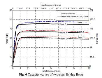
Extra information on the comparison of the analytical results with the test data, which confirmed the adequacy of the computer model in reproducing two-span RC bridge responses, can be found in the work of Sadrossadat Zadeh et al. (2007).
