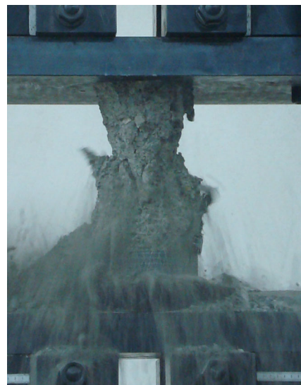
Fig. 7. Abrupt failure mode of FRP strengthened specimen
