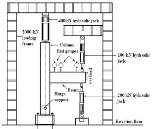
Fig. 4 Schematic Experimental Test Setup
