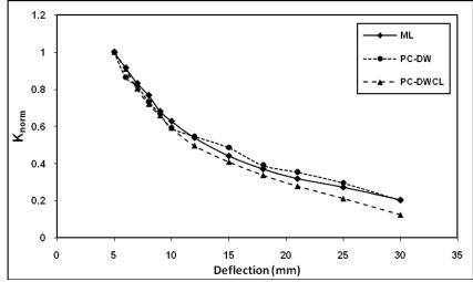
Fig. 14 Normalized Stiffness Degradation of the three specimens
