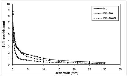
Fig. 13 Stiffness Degradation of three specimens
