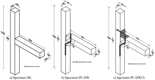
Fig. 3 Isometric views of a) Specimen ML, b) Specimen PC-DW and c) Specimen PC-DWCL
