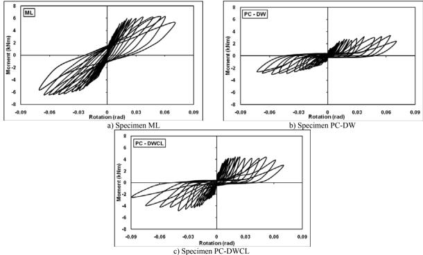
Fig. 9 Hysteresis Moment-Rotation curves of all the specimens
