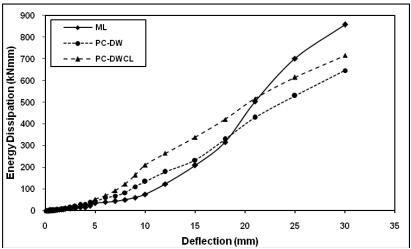
Fig. 11 Cumulative energy dissipation curves of the three specimens
