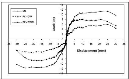
Fig. 10 Load-displacement envelopes of specimens ML, PC-DW and PC-DWCL
