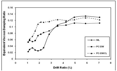
Fig. 12 Equivalent Viscous Damping Ratio curves of the three specimens
