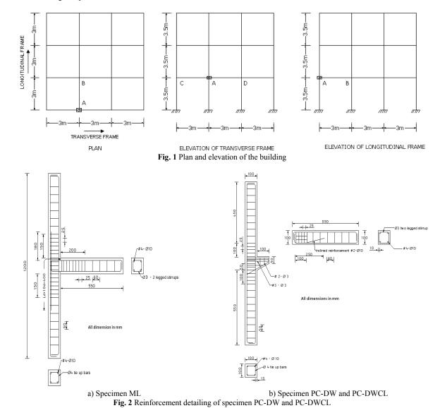
4.3. Test specimen and connection details
