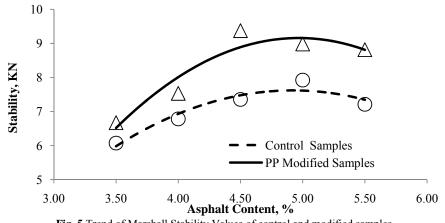
Fig. 5 Trend of Marshall Stability Values of control and modified samples
