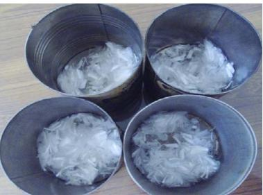
Fig. 2 Polypropylene fibres taken in containers
