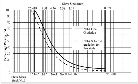
Fig. 1 Aggregate gradation curve
