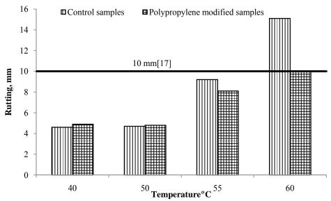
Fig. 6 Average final rut depths of control and modified samples
