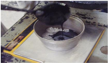
Fig. 3 Mixing asphalt binder and fibres
