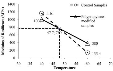
Fig. 8 Temperature and IDT strength correlation for control and modified samples
