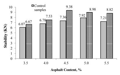
Fig. 4 Marshall Stability of control and modified samples
