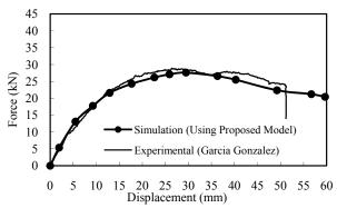
Fig. 11 Comparison of simulated results using the proposed model and experimental tests of Garcia Gonzalez [5],  $\Omega = 45^{\circ}$
