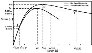
Fig. 1 Proposed stress-strain curves for confined and unconfined concretes under monotonic loading (Envelope curve for cyclic loading
