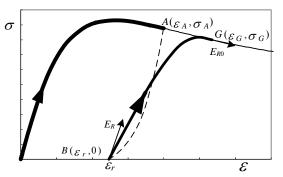
Fig. 5 Reloading from a point of zero stress
