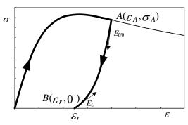
Fig. 2 Unloading from the envelope curve
