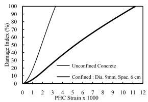
Fig. 15 Microscopic damage index, calculated for confined and unconfined concretes under cyclic loading
