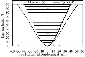
Fig. 17 Macroscopic Damage index, calculated for tested columns under cyclic and monotonic loading
