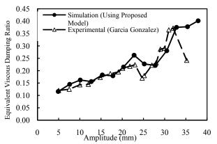
Fig. 14 Comparison of equivalent viscous damping ratio when using the proposed model and experimental tests [5], cyclic loading,  $\Omega = 30^{\circ}$
