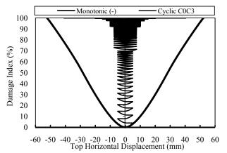
Fig. 18 Meyer's Damage index, calculated for tested columns under cyclic and monotonic loading
