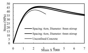
**Fig. 7** Effect of the spacing of transverse reinforcements,  $f_c' = 42$  MPa
