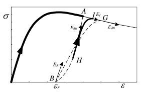
Fig. 6 Reloading from a point on the unloading trajectory
