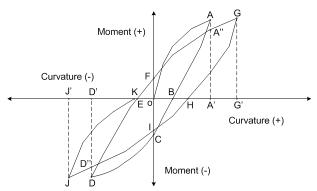
Fig. 16 Schematic illustration of damage index "D" calculation procedure for cyclic loading
