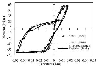
Fig. 12 Comparison of simulated results using the proposed model and experimental tests and simulation of Park [6]
