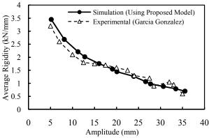
Fig. 13 Comparison of the average rigidity when using the proposed model and experimental tests [5], cyclic loading,  $\Omega = 30^{\circ}$
