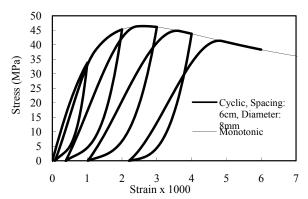
**Fig. 8** An example of the application of the proposed stress-strain model,  $f_c' = 42 \text{ MPa}$
