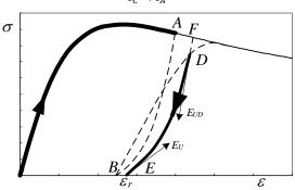
Fig. 4 Unloading from a point D on the reloading curve when  $\varepsilon_D > \varepsilon_A$
