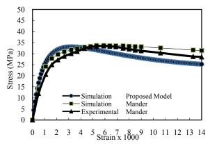
Fig. 9 Comparison of the proposed model with experimental tests and simulation of Mander [23]
