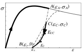
Fig. 3 Unloading from a point C on reloading curve when  $\varepsilon_C < \varepsilon_A$
