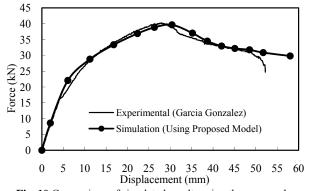
Fig. 10 Comparison of simulated results using the proposed model and experimental tests of Garcia Gonzalez [5],  $\Omega$  = 0°
