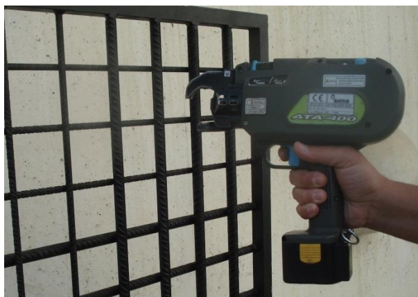
Fig. 6 Battery powered rebar tier
