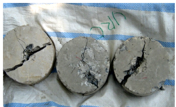
Fig. 2b Steel fibrous concrete disc specimens after failure
