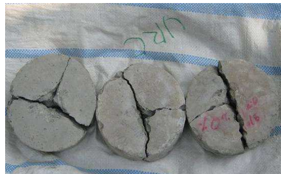
Fig. 2a Non-fibrous (silica fume) concrete disc specimens after failure
