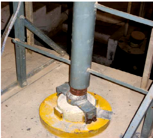
Fig. 1 Disc specimen under drop weight impact test
