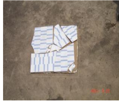
Fig. 5 Expanded polystyrene with saw dust and broken glazed tiles
