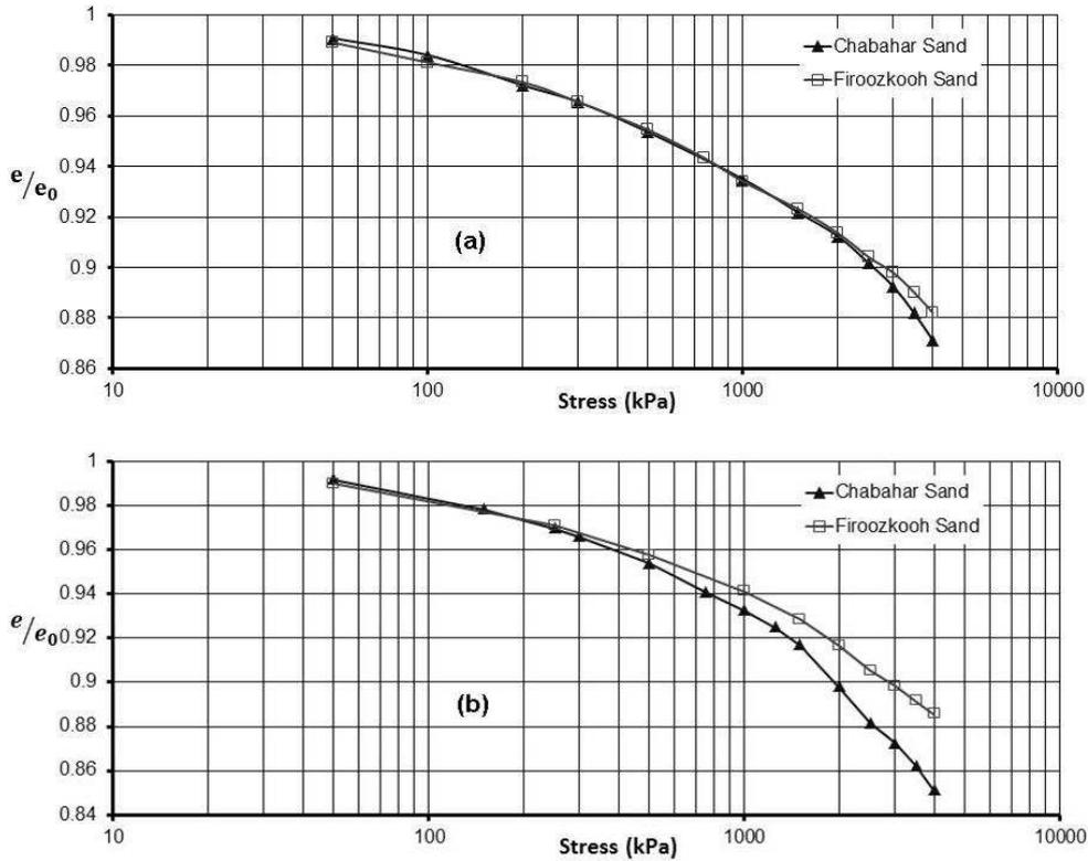
Fig. 4 Normalized void ratio versus normal stress: (a) densely packed samples, (b) loosely packed samples
