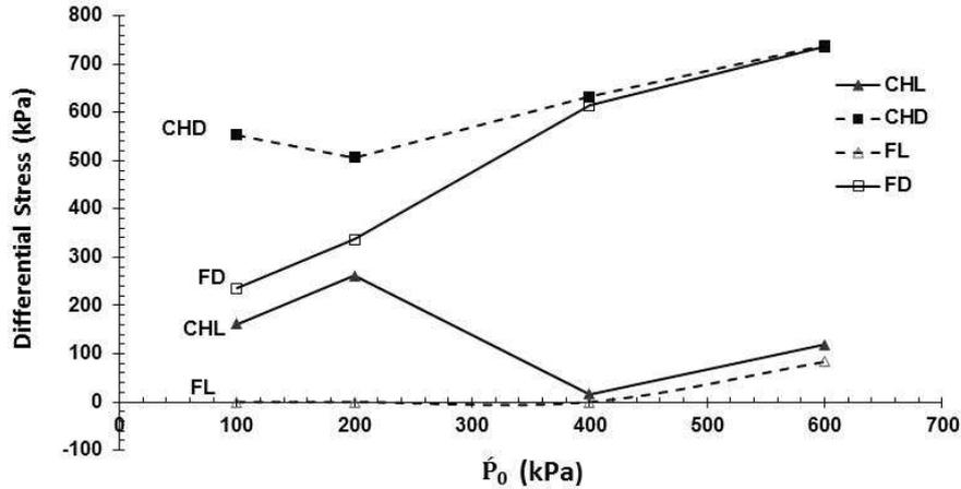
Fig. 8 The discrepancy between the shear strengths ( $q$ ) at the peak point and end of the test (axial strain 20%)
