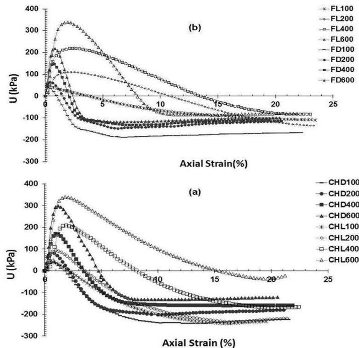
Fig. 9 Changes of excess pore water pressure versus axial strain: (a) Firoozkooh sand, (b) Chabahar sand
