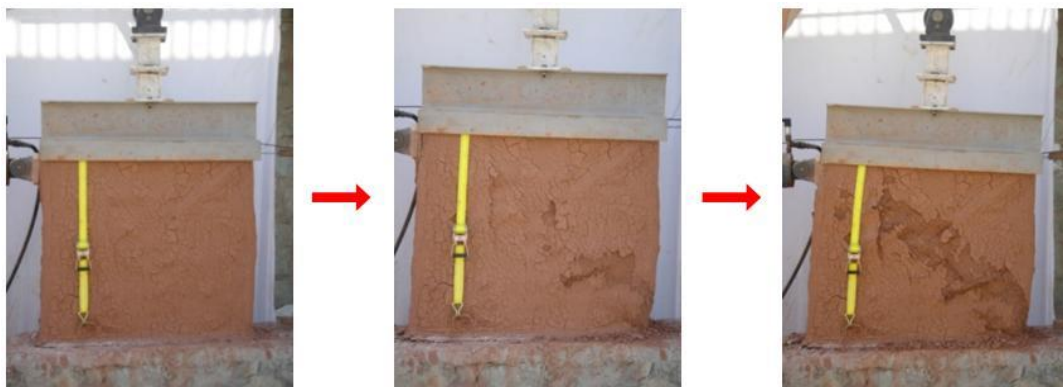
Fig. 18 Damage mechanism of RMW2 wall
