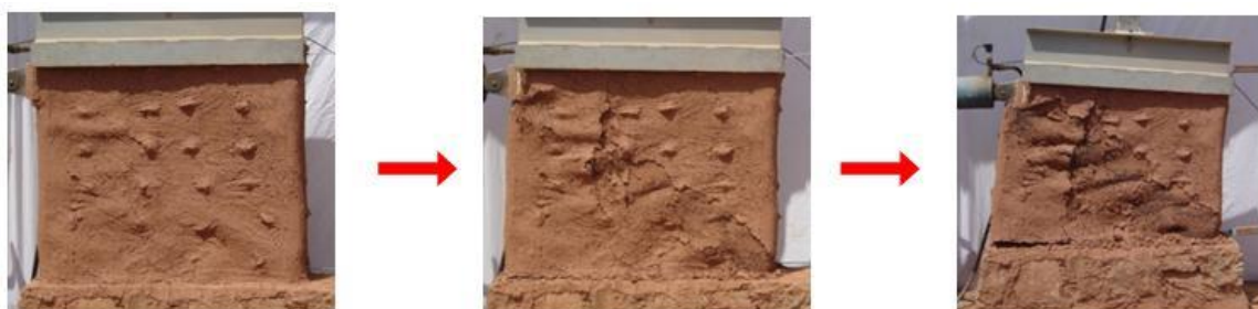
Fig. 15 Damage mechanism of RMW1 wall
