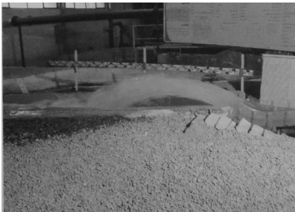
Flip Bucket Model of Jareh Dam
