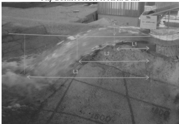
Flip Bucket Model of Ajab Shir Dam
