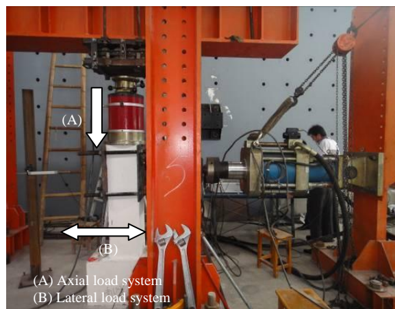
Fig. 3 Test set-up for cyclic loading test
