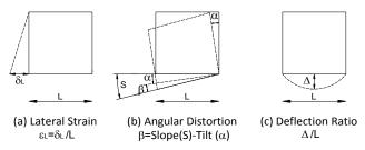
Fig. 2 Deflection parameters used in damage criteria
