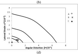
Fig. 12 (a) Ground surface settlement, (b) Deformation of excavation wall, (c) Strut stress during excavation procedure, (d) Deflection parameters of building in Boscardin and Cording diagram
