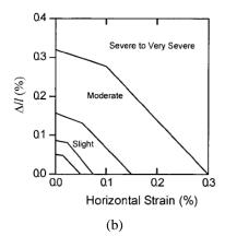
Fig. 3 Damage level a) in relation to  $\beta$ ,  $\varepsilon_l$  (Boscardin and Cording 1989), b) in relation to horizontal strain,  $\Delta L$  (Burland 1995)
