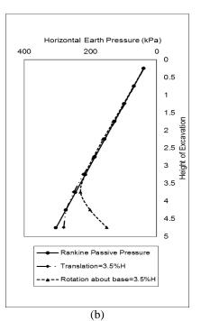
Fig. 6 Comparison Rankine closed form solutions with numerical model simulating (a) active and (b) passive retaining wall
