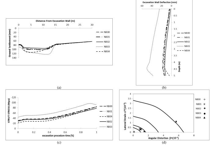
Fig. 11 (a) Ground surface settlement, (b) Deformation of excavation wall, (c) Strut stress during excavation procedure, (d) Deflection parameters of building in Boscardin and Cording diagram
