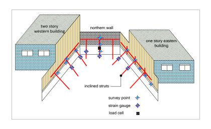
Fig. 8. 3D view of excavation and instrumentation
