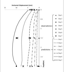
**Fig. 9.** Comparison of northern wall deflections between observations and numerical results at excavation days
