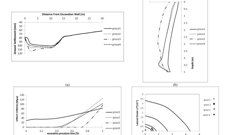
Fig. 14 (a) Ground surface settlement, (b) Deformation of excavation wall, (c) Strut stress during excavation procedure, (d) Deflection parameters of building in Boscardin and Cording diagram
