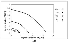
Fig. 15 (a) Ground surface settlement, (b) Deformation of excavation wall, (c) Strut stress during excavation procedure, (d) Deflection parameters of building in Boscardin and Cording diagram
