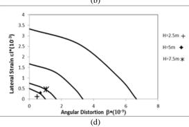
Fig. 13 (a) Ground surface settlement, (b) Deformation of excavation wall, (c) Strut stress during excavation procedure, (d) Deflection parameters of building in Boscardin and Cording diagram
