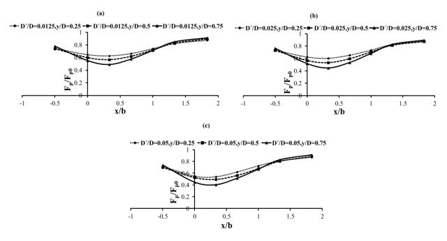
Fig. 14 Effects of the drain position on uplift force (  $\frac{H}{D}$  = 0.5 )
