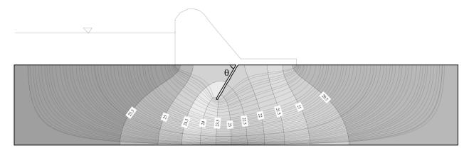
Fig. 7 Results from the numerical model for the inclination angle of 60 degrees
