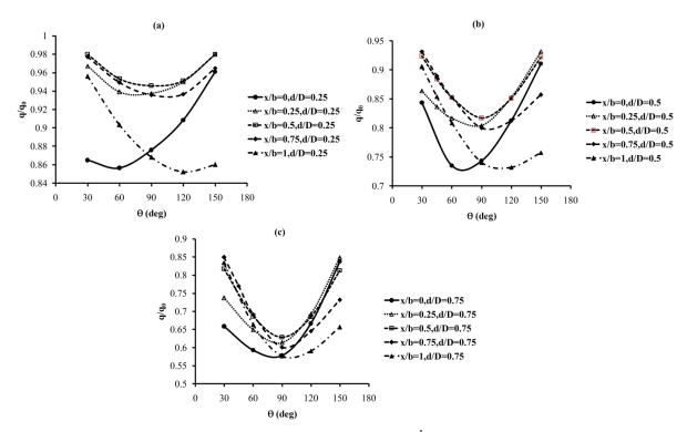
Fig. 8 Effect of Cutoff wall situation and inclined angle on seepage discharge for  $\frac{h}{D} = 0.25$  (a)Short cutoff wall, (b) Medium cutoff wall, (c) Long cutoff wall
