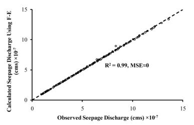
Fig. 2 Evaluation of F-E method for estimating a) Uplift force, b) Unit seepage discharge
