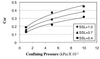
Fig. 7 Coefficient of stress recovery (Csr) versus confining pressure for dry-saturated tests
