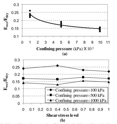
Fig. 13 Ratio of the material elasticity modulus under saturated condition to the elasticity modulus under dry condition ( $E_{wet}/E_{dry}$ ), a) versus confining pressure, b) versus shear stress level
