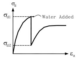
Fig. 6 Typical behavior of dry-saturated specimens
