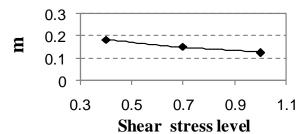
Fig. 8 Coefficient m versus shear stress level for dry-saturated
