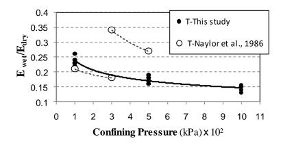
Fig. 16 Comparison of the variation of E<sub>wet</sub>/E<sub>dry</sub> against confining pressures, obtained from this study and another investigations
