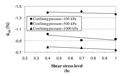
Fig. 11 Change in volumetric strain due to saturation ( $\mathcal{E}_{vc}$ ), a) versus confining pressure, b) versus shear stress level.
