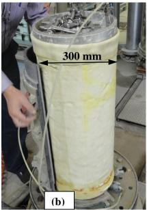
Fig. 1 (a) Testing material separated based on individual sieve size (b) prepared specimen
