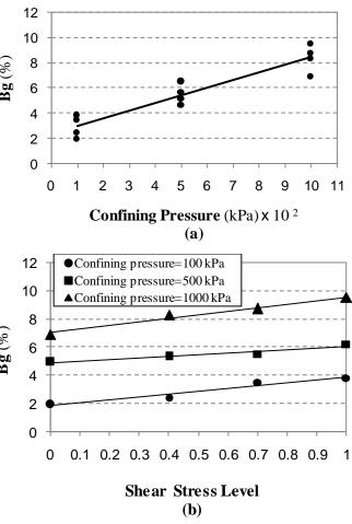
Fig. 17 Particle breakage index, Bg, a) versus confining pressure, b) versus shear stress level.
