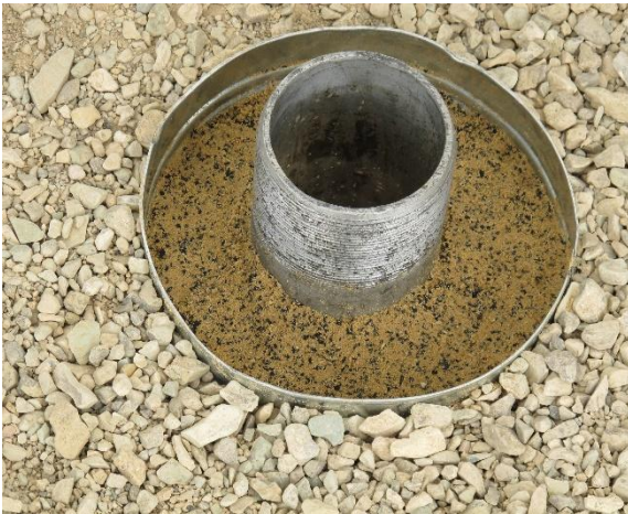
Fig. 10 Preparing the Soil-Rubber Mixture and Constructing Iso_M Model
