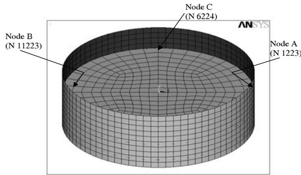
Fig.1 finite element mesh for liquid filled tank
