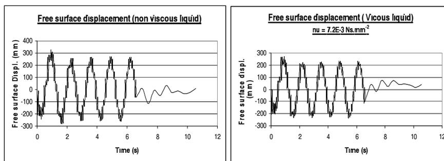
**Fig.12** effect of liquid viscosity on sloshing amplitude
