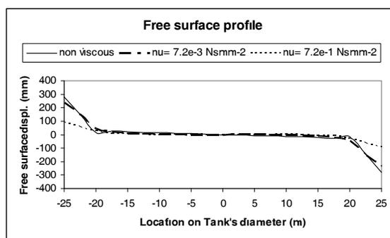
**Fig.13** effect of liquid viscosity on sloshing profile
