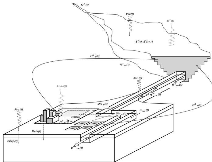
**Fig. 1** Typical scheme of Cyclic Storage (CS) system.
