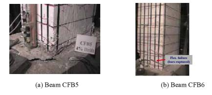
Fig.6 Observed Damages in Beams CFB5 and CFB6
