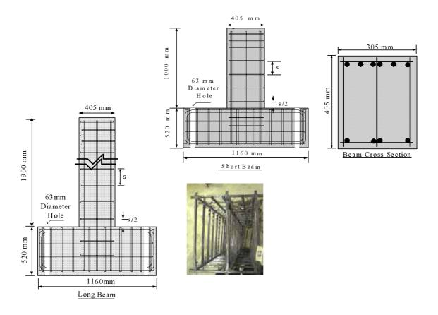
Fig.1 Geometry of Cantilever Beams
