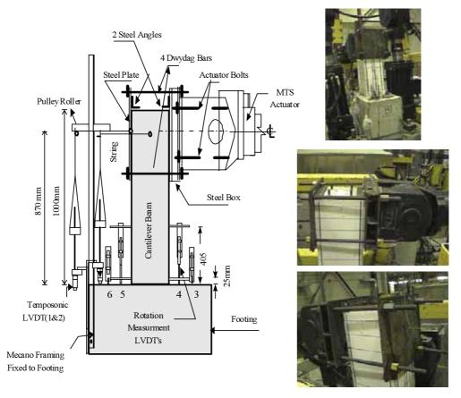
Fig.3 Locations of LVDT's and the Test Setup for Beams
