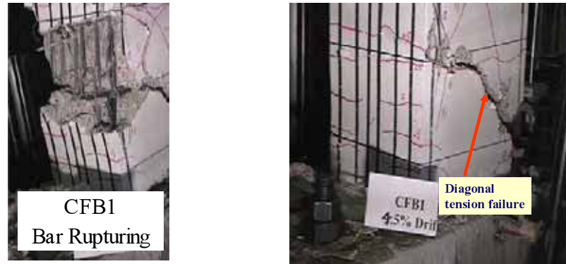
Fig.4 Observed Damages in Beam CFB1
