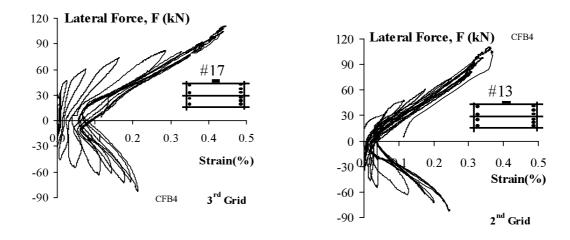
Fig.8 Grid Strain Readings in Beams
