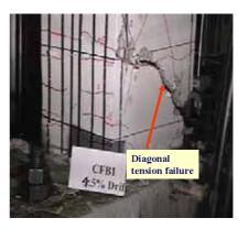
Fig.4 Observed Damages in Beam CFB1
