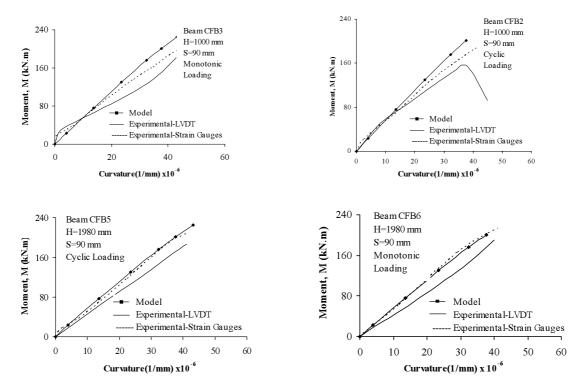
Fig.13 Moment-Curvature Diagrams of Beams
