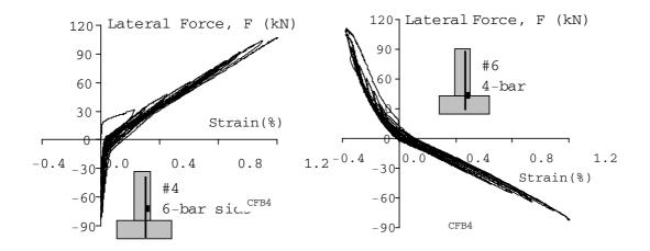
Fig.7 Bar Strain Readings in Beams
