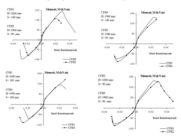
Fig.11 Moment-Total Rotation Relationships of Beams
