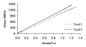
Fig.2 Tensile Stress-Strain Relationship of Pultrall CFRP Bars
