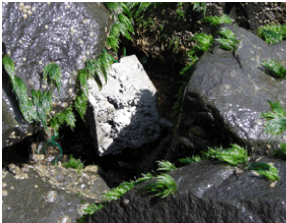
Fig. 2. shows the natural culture of the marine algae Ulva fasciata on concrete cube
