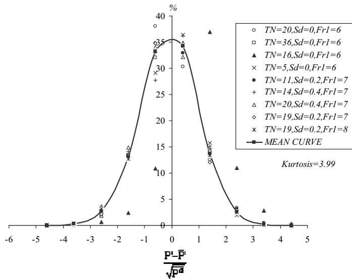
Fig. 11. Probability density distributions of pressure fluctuation
