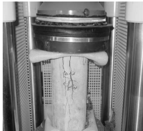
Fig.6 Cylindrical sample under compression test
