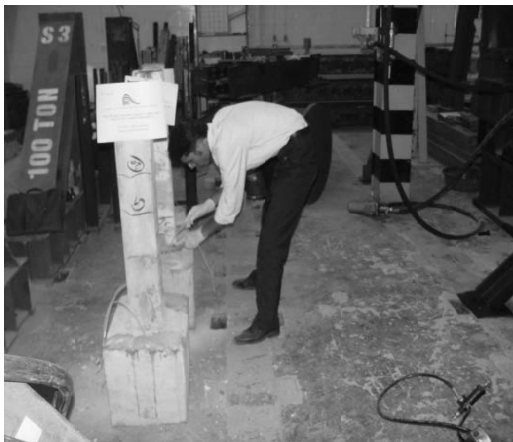
Fig.8 Cleanig surface of the damaged columns
