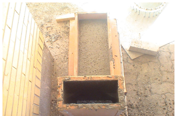
Fig. 5. L-box test of SCLWC
