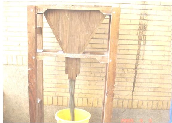
Fig. 4. V-funnel test of SCLWC
