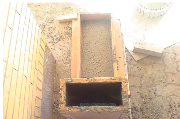
Fig. 5. L-box test of SCLWC
