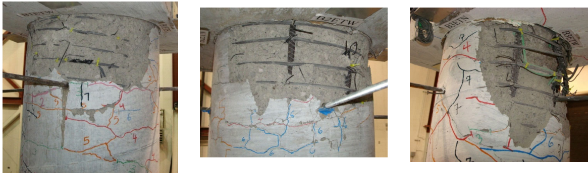
Fig. 7. Upper plastic hinge after final motion: left to right, SMA pier, PT pier, and ISO pier
