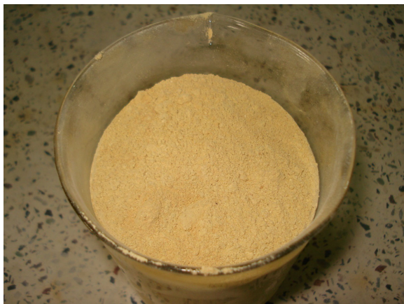
Fig. 3. Dried and Pulverized Electroplating Waste Sludge after Treatment and Precipitation
