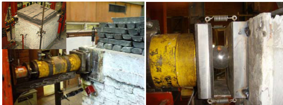
b) Application of loading system
