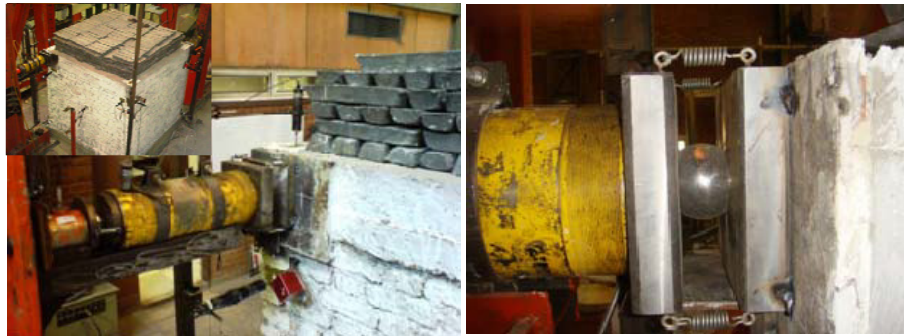
b) Application of loading system
