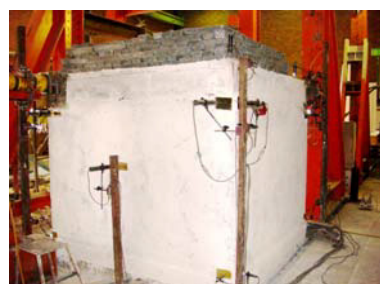
d) Instrumented specimen ready for test
