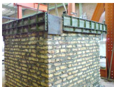
c) Reinforcing and concreting of slab and upper tie
