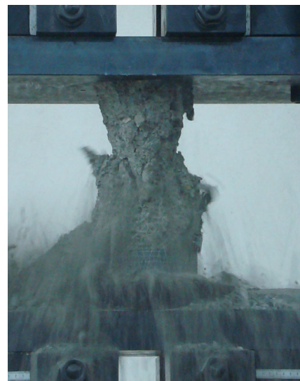
Fig. 7. Abrupt failure mode of FRP strengthened specimen
