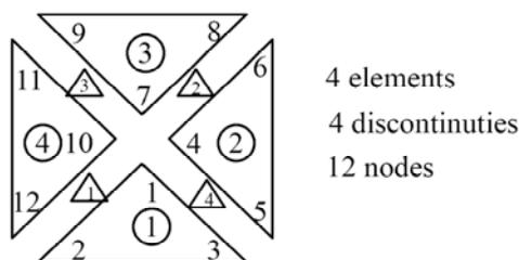
Fig. 1. Triangular element mesh for dynamic Shakedown analysis [11]
